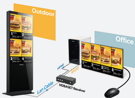
Figure 8. Remote management of outdoor signage with simple, low-cost connection through advanced HDBaseT
